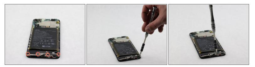
Once the back has been removed, you will need to unscrew the four screws on the bottom panel with an AT3 bit.
