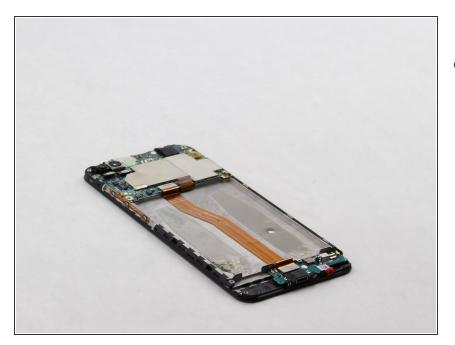
Remove the battery and replace it with the new battery.
