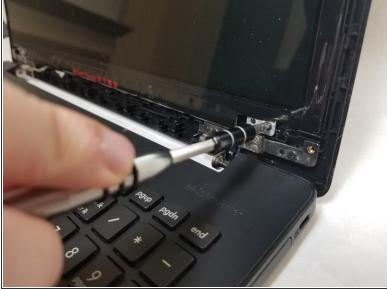
• Use a JIS #0 screwdriver to unscrew the four 3.5mm screws.
