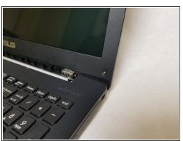
Use a JIS #0 screwdriver to remove the two 4.5mm screws.
