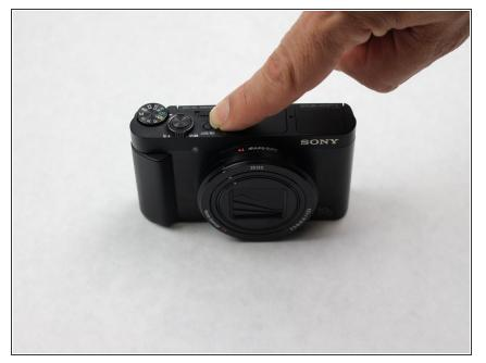
Before disassembling any part of the camera, turn off power by pressing down on the ON/OFF button. The ON/OFF button is located on top of the camera.
