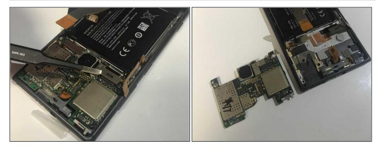
• Remove the motherboard by sliding tweezers between it and the back of the screen. Lift up.
