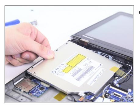
Slide the optical drive away from the motherboard in order to remove it.
