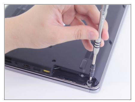
• Remove the M3 x 2mm screw from the hole left by the hard drive using a Phillips #00 screwdriver.
