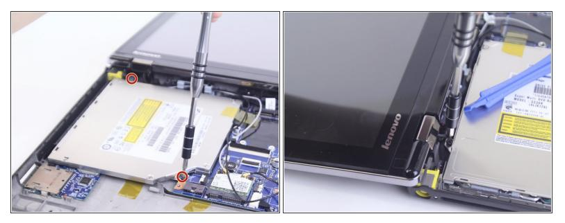
Remove the two M2 x 3mm securing the the optical drive to the device using a Phillips #000 screwdriver.
