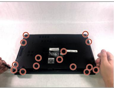
After removing the battery, remove 15 7mm screws using the Phillip #1 Screwdriver.
