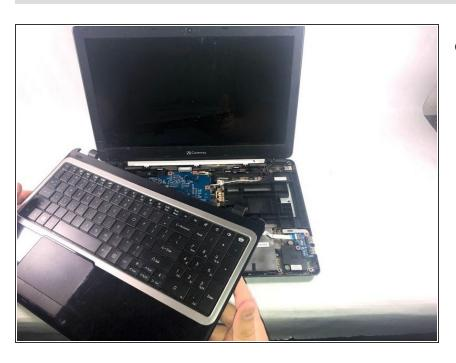
Lift the upper case cover off of the device. Use a prying tool along the edges if necessary.
