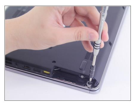
Remove the M3 x 2mm screw from the hole left by the hard drive using a Phillips #00 screwdriver.
