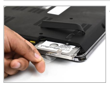
Use the clear tab to slide the hard drive out of the device.
