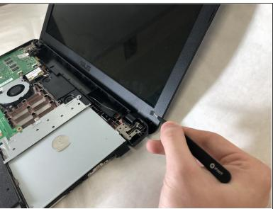
• Use tweezers to remove small plastic screw covers from the bottom corners of the screen.
