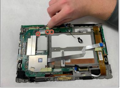
Detach the Wifi and GPS antennas (three coaxial cables connected to the motherboard) using hands, metal spudger, or tweezers by lifting away from the device.
