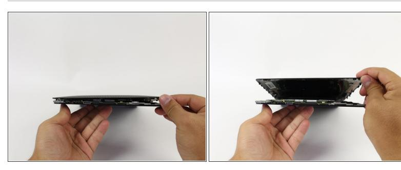
Remove back panel by pulling away from the remaining device.
