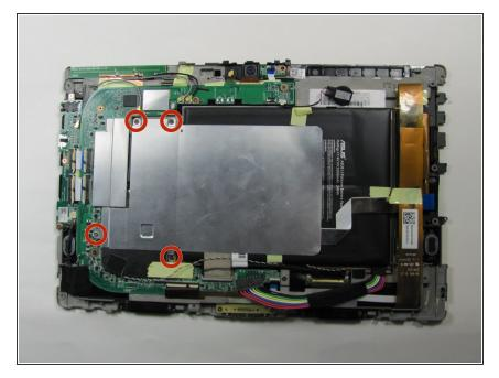
Use Phillips #00 Screwdriver to remove four 3 millimeter screws found on the metal panel.
