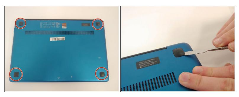
• Using the metal spudger, remove all the rubber squares on the bottom of the laptop.
