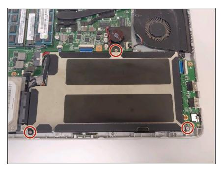
Remove the three 3mm screws located on the perimeter of the battery using the Phillips #1 screwdriver.
