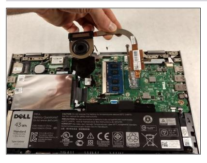
Grasp the fan and lift upward.
