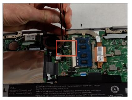
Use the <u>tweezers</u> to gently pull the power supply cable from its port.
