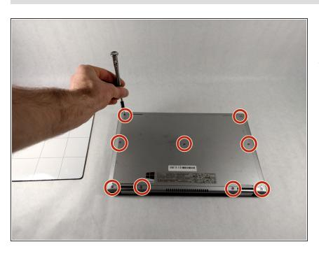
Using the Phillips #1 screwdriver, remove all nine 7mm screws.
