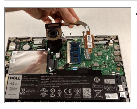
Grasp the fan and lift upward.
