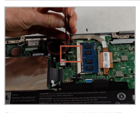
Use the tweezers to gently pull the power supply cable from its port.
