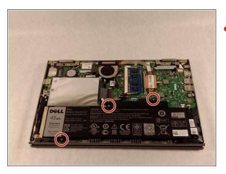
Remove the three 4mm screws holding battery in place using the Phillips #0 screwdriver.
