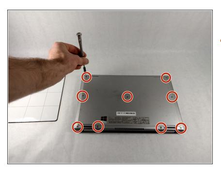
Using the Phillips #1 screwdriver, remove all nine 7mm screws.
