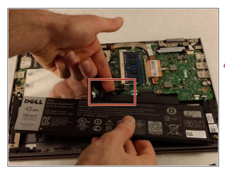
Once loosened, use your fingers to lift the battery up and out of its housing.
