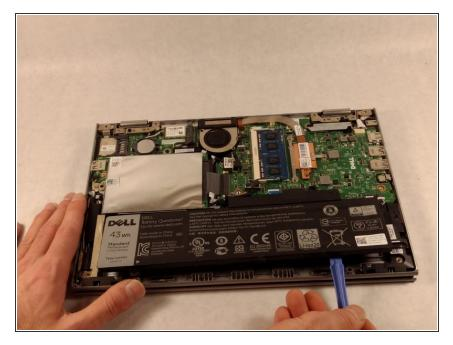
• Using the iFixit opening tools, lift the battery out of its housing.
