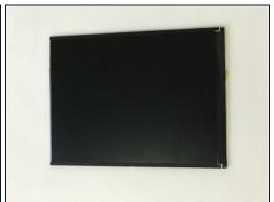
Use the suction cup to loosen and pull up the screen.
