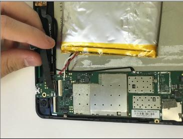
Remove all wire connections by sliding them out of the connectors.
