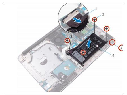
Remove the screws that secure the battery to the palm rest and keyboard assembly.
