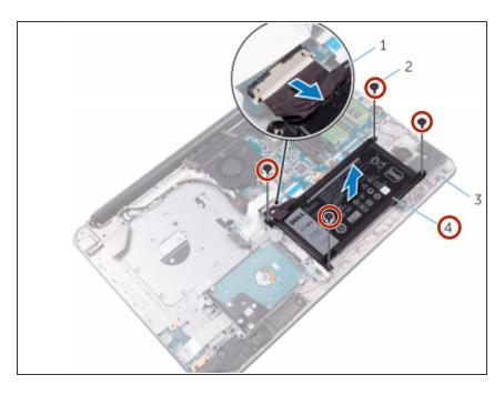
Align the screw holes on the battery with the screw holes on the palm rest and keyboard assembly
