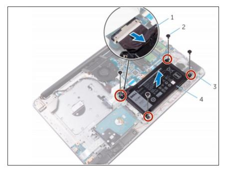
Replace the screws that secure the battery to the palm rest and keyboard assembly.
