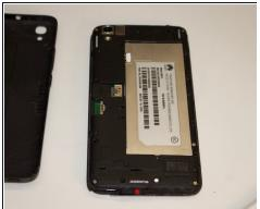
Use the opening tool from the iFixit kit to get under the back cover and, gently separate the back from the front.
