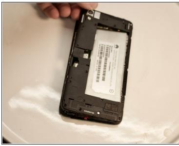
Remove the 15 screws on the back of the phone with a Phillips #000 screwdriver.
