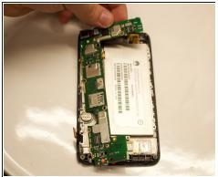
• Disconnect the connectors from the motherboard and gently remove the motherboard.
