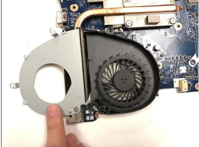
Remove the six 2mm Phillips #00 screws.
