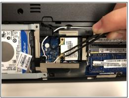
• Remove the back panel, and remove the white cable from the wifi chip using a pair of tweezers.
