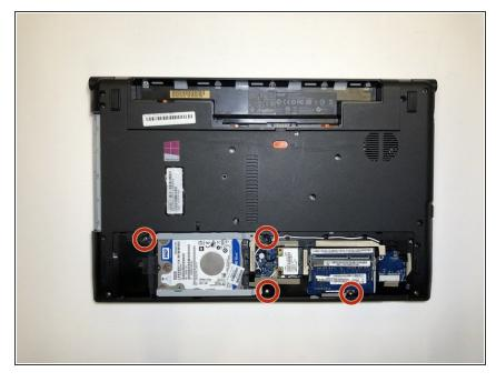
Using a Phillips head #0 screwdriver, remove the four 5.3 mm screws.
