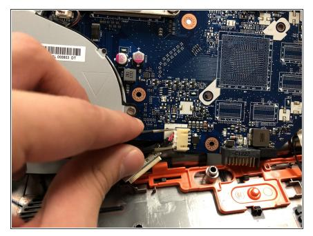
Flip the motherboard over and using a pair of tweezers, remove the cable.
