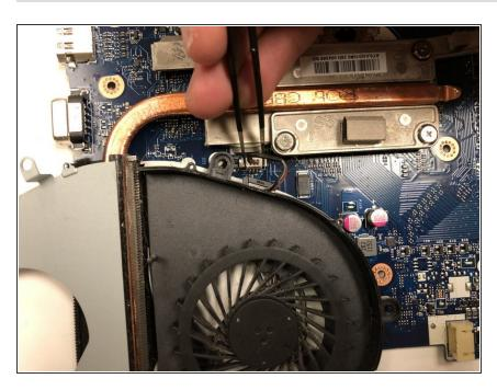
Using a pair of tweezers, remove the cable.
