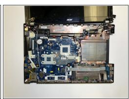
Flip the computer over and remove the touchpad cover and keyboard.
