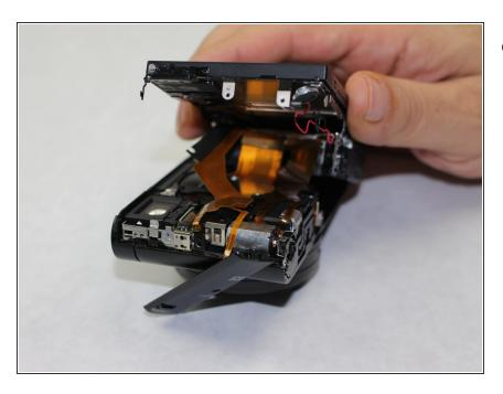
After loosening the plastic edges of the camera, gently pull the LCD screen upwards.
