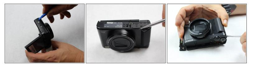
• Use the plastic opening tools included in the iFixit tool kit first. If the shell/parts do not detach from each other, use metal spudgers as a last resort to loosen/separate the plastic shell of the camera. Keep in mind that there may be more screws holding parts together. Work delicately and separate sides evenly.
