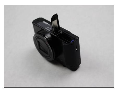
• Open the compartment located at the bottom of the camera. Slide the LOCK/OPEN switch to the OPEN side. Locate the small blue tab on the side. Pull it in the direction away from battery. Remove the battery and set it aside.
