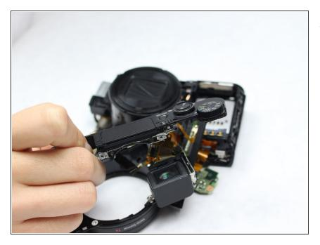
• Replace the non-functioning top piece of the camera with a new one.
