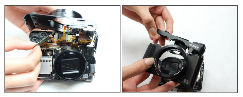
• Gently pull the circuit board off the top piece. The top piece, which has the shutter button attached, will then be detached from the rest of the camera.
