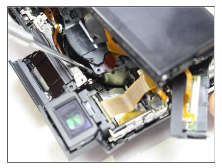
• Use metal spudger to detach the face of the screen off the rest of the camera. Be extremely careful as there is a thin golden film/plastic ribbon holding the face of the screen to the rest of the camera.
