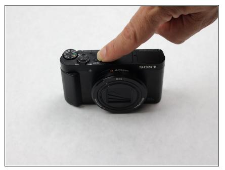
Before disassembling any part of the camera, turn off the power by pressing down on the ON/OFF button. The ON/OFF button is located on top of the camera.
