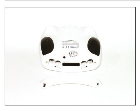
Pull the plastic piece off to reveal the compartment where the batteries go.
