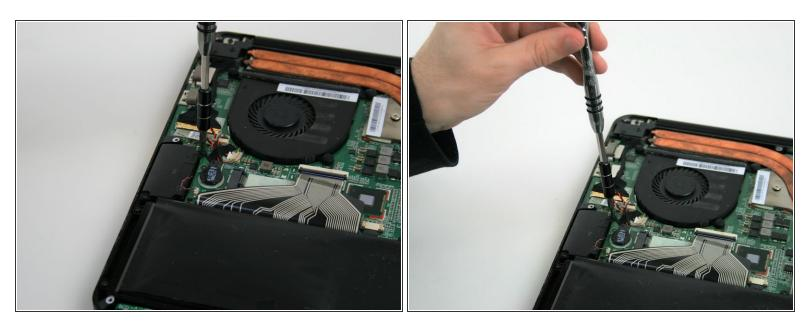
• Using a Phillips #0 screwdriver, remove the two screws holding down the speaker.
