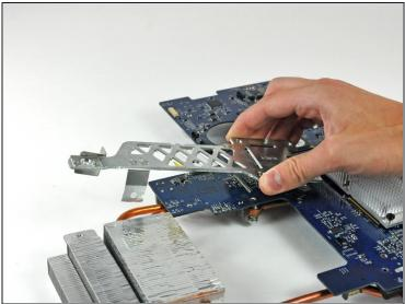
• Carefully lift both metal heat sink brackets off the logic board.
