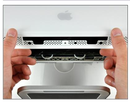
While holding the RAM arms in with your thumbs, lift the lower edge of the front bezel enough to clear the rear case.
