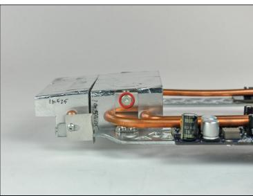
• Remove the 6.1 mm T8 Torx screw from both sides of the heat sink nearest the logic board (two screws total).
