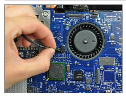
Disconnect the optical drive thermal sensor cable from the logic board by pulling its connector toward the left edge of the iMac.
