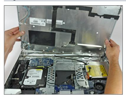
While holding the display perpendicular to the rear case, pull it upward to peel off the EMI shield stuck to its upper edge.
