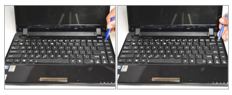
Use a plastic opening tool and carefully pry the top panel from the base.
