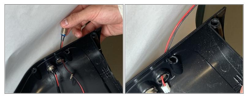
Remove the power button from the hoverboard assembly.
