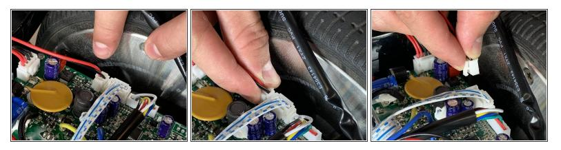
Unclip the red and black power cables that are attached to the port from the motherboard.
