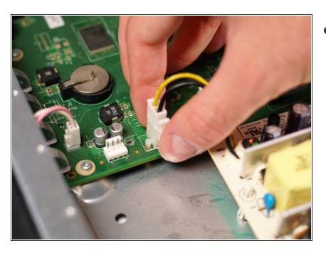
Remove the power supply wire by pinching the plastic connection and gently pulling away from the motherboard.
