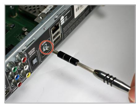
Remove the single 80 mm T10 screw above HDMI port using the Torx screwdriver.
