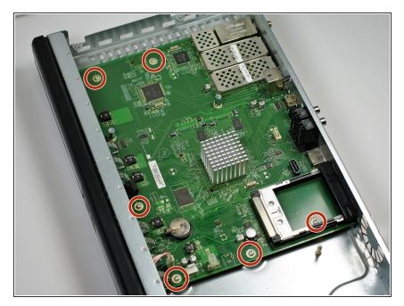
Remove the six 80 mm T10 screws using the Torx Screwdriver.
