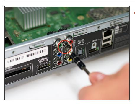
Remove the single 140 mm T8 screw from the back panel using a Torx screwdriver.
