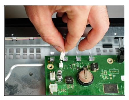
Remove wire connected to the front of of the box by pinching the connector and gently removing from the motherboard.
