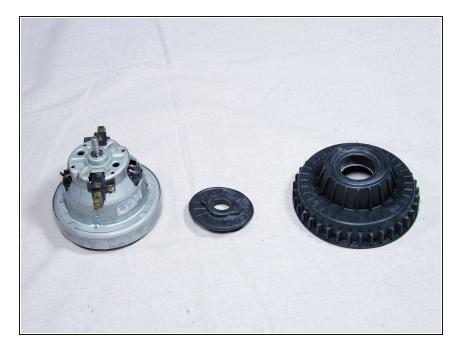
• Remove the two rubber grommets from your old motor, then transfer them to your new motor.
