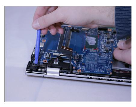
Use the iFixit opening tools to pry motherboard from back of laptop.
