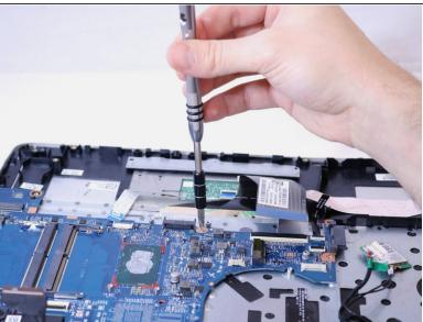
Use a PH1 screwdriver to unscrew six 3 mm Phillips head screws on the motherboard.
