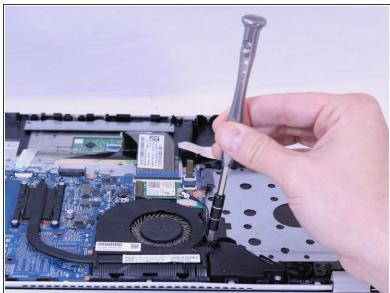
• Use a PH0 screwdriver to unscrew the three 3 mm Phillips head screws located on the fan.
