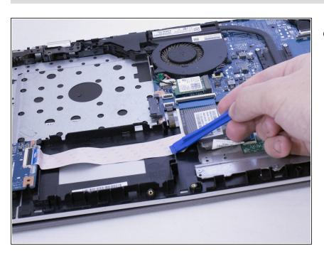
Lift the plastic wedges up on both sides of the hard drive.
