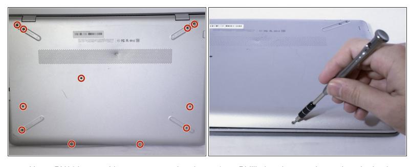
Use a PH000 screwdriver to unscrew the eleven 4mm Phillip head screws located on the back panel.
