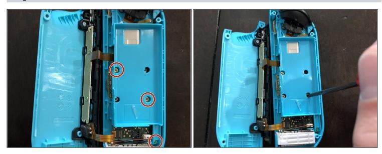
• Use a Phillips #2 screwdriver to remove the three screws that are locking the inner casing into place.
