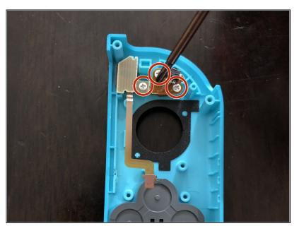
Using a Phillips #2 screwdriver, remove the three screws holding the minus button and L button into place.
