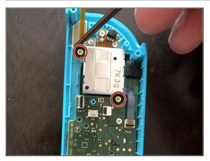
Using a Phillips #2 screwdriver, unscrew both screws connecting the analog stick to the motherboard.
