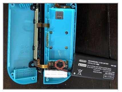
Gently pull the cord that's connecting the battery to the motherboard up and out of the Joy-Con.
