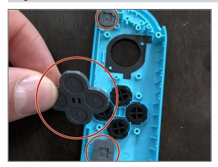
Locate and remove all of the rubber casings covering the buttons.
