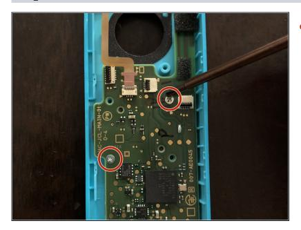
Using a Phillips #2 screwdriver, remove the two screws holding the motherboard in place.
