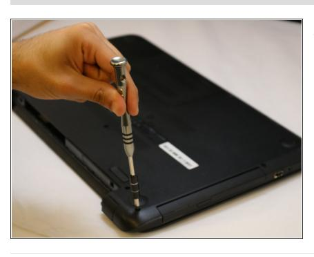
Start take out the screws to open the laptop cover and replace the DVD plug. Use Phillips screwdriver Flathead 2.5 mm
