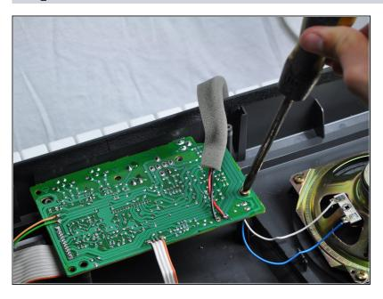
Once the wires are firmly attached, screw the circuit board back into the keyboard.
