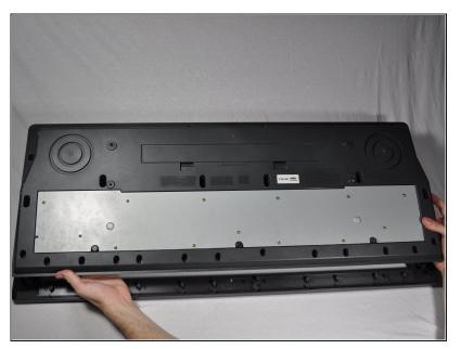
Remove the bottom panel by lifting and pulling it towards yourself.
