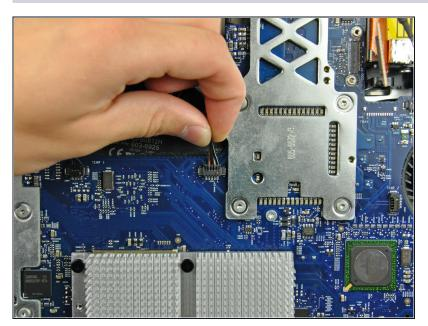
Disconnect the CPU fan from the logic board by pulling its connector toward the top edge of the iMac.
