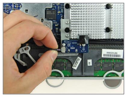
Disconnect the IR board cable by pulling its connector away from the socket on the IR board.
