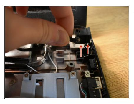
Follow the cable to the power jack port and carefully lift up to remove it from the laptop.
