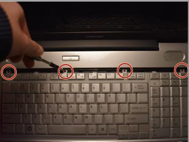
Remove the four screws using the Phillips #1 screwdriver.
