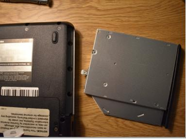
Gently slide the optical drive out of the device.
