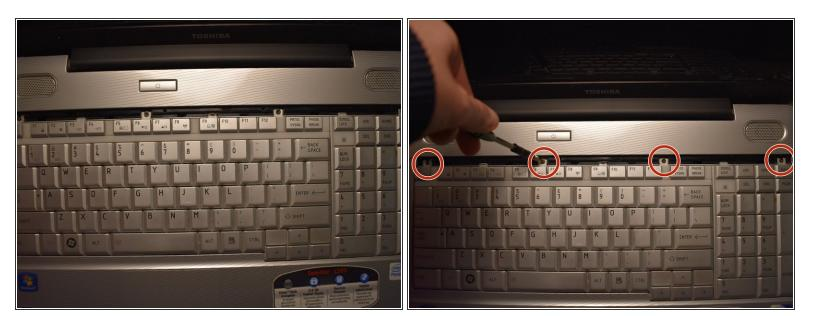
• Remove the four screws using the Phillips #1 screwdriver.
