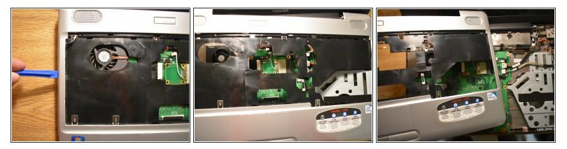
• Using the opening tool, carefully go around the edge and loosen the palm-rest assembly, until you can comfortably and easily lift it off.
