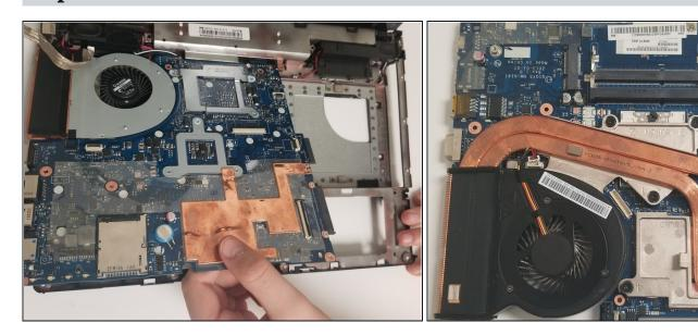
• After unscrewing the screws, remove the motherboard.
