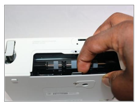
• Make sure the metal tab on the printer will fit over the paper in the Cassette.
