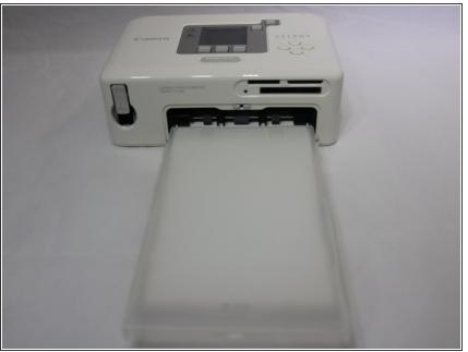
This configuration allows printing but not reloading of the paper cassette.
