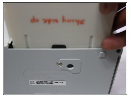
Push the cassette into the printer, with the glossy side up. Make sure that the Cassette is being guided by the studs in the mouth of the printer.
