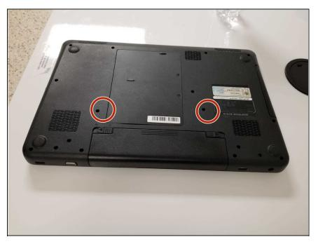
Remove both screws that connect the keyboard to the laptop chassis.
