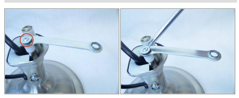
• Using a Phillips #3 screwdriver, unscrew the 15 mm long bolt fastening the oscillation arm to the fan base bolt.
