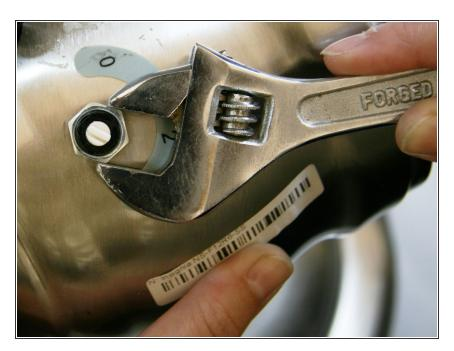
Unscrew the flat 17 mm nut fastened at the bottom of the power knob with a small crescent wrench.
