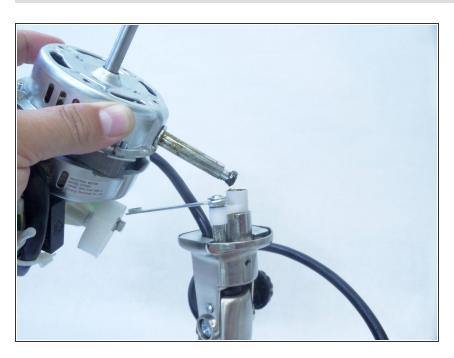
Remove the fan motor assembly from the base.
