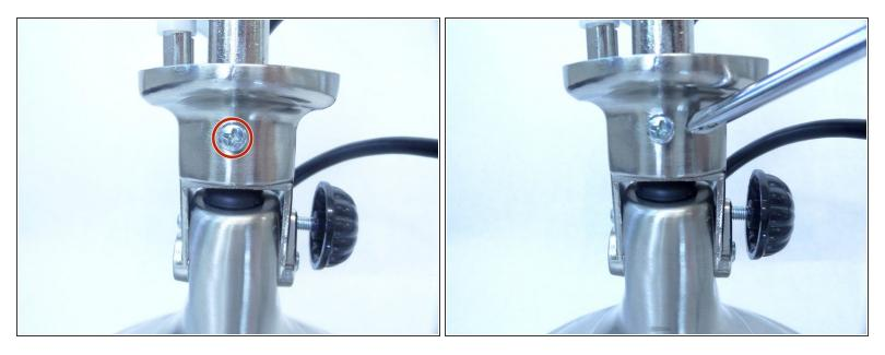
Using a Phillips #3 screwdriver, unscrew and remove the 4 mm long bolt on the front face of the base that fastens the motor assembly to the base bolt.
