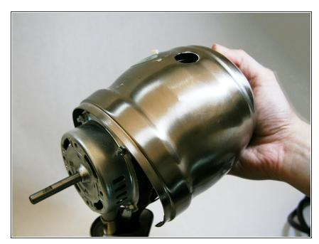
Slide the back end of the motor housing away from the front of the rotor.
