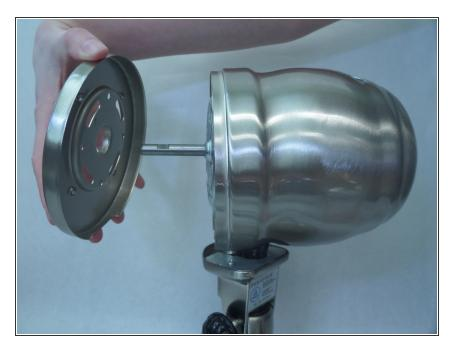
Pull the front face of the motor housing off toward the front of the rotor.
