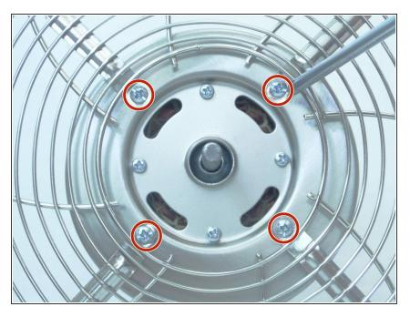
Unscrew the four 8 mm bolts that fasten the back of the fan cage back to the motor housing with a Phillips #3 screwdriver.
