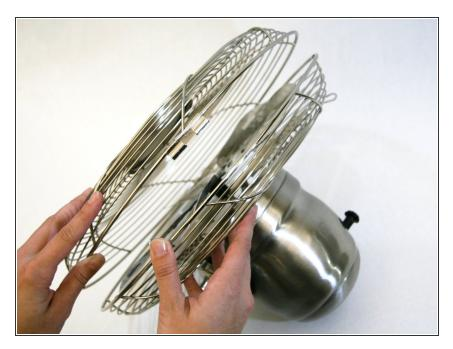
Remove the front of the fan cage.
