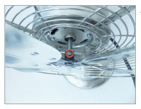
Remove the 8 mm bolt fastening the fan blades to the rotor with a Phillip #3 screwdriver.
