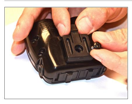
When installing the mount, line the hole in the device with that of the mount and screw into place.
