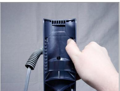
Push outward on the two plastic clips that secure the switch cover to the vacuum.
