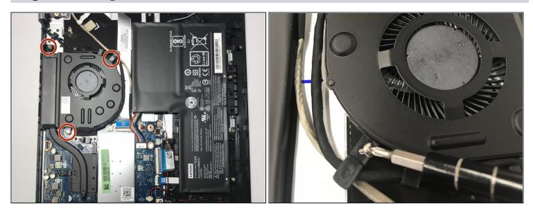
• Remove the three 5mm screws using the T5 Torx Screwdriver.
