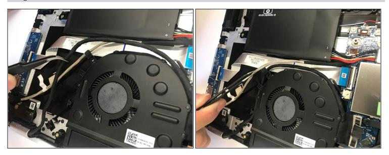
• Pull black wire and gray wire away from cooling fan clips using the tweezers.
