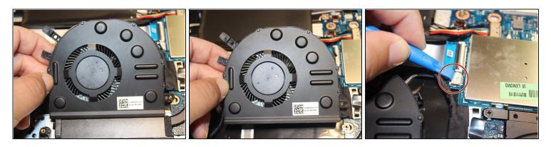
• Pull out the cooling fan from where it is attached and pull it up until you see where the wire is attached to the motherboard. Using the iFixit Opening Tools, detach the connector.
