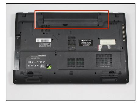
Turn over the laptop so the battery compartment is facing up.
