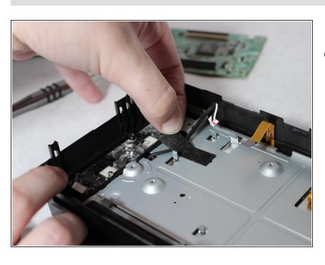
Carefully remove the tape attaching the power cable to the metal plate.
