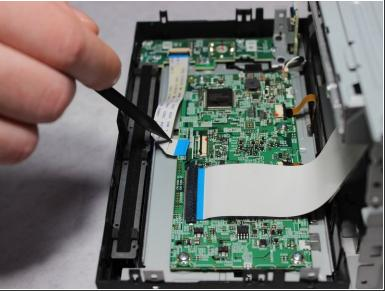
• Flip up the black clasp with the spudger to disconnect the small white ribbon cable from the main board.
