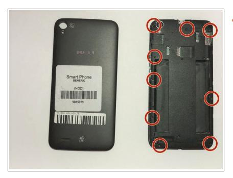
Remove all the nine 2mm screws using the JIS #00 Screwdriver.
