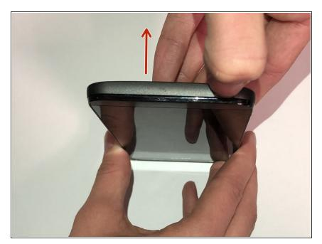
Pry the back cover from the bottom of the phone, pulling outwards and upwards.
