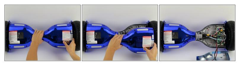
• Grip the bottom left panel and lift up to remove.
