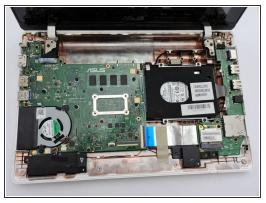
Gripping the wider left section, lift the battery up and away from computer.
