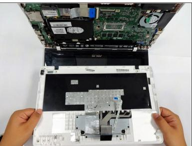
Now that the keyboard connectors are unplugged, pull the keyboard off and away from the back panel hinges.
