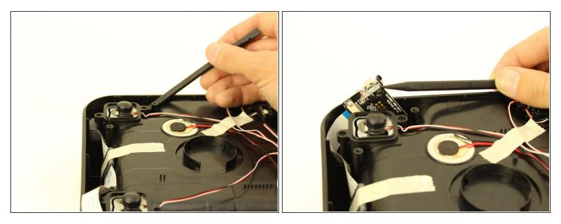
• Use the nylon spudger to remove the charging assembly from the SmartBowl.
