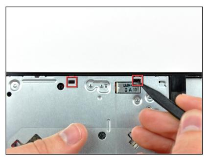
Use the tip of a spudger to push the two optical drive bracket tabs out of their slots in the top of the optical drive.
