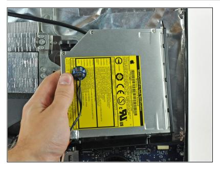
Maneuver the optical drive out of the rear case, minding the two plastic pins molded into the rear case near the open end of the optical drive that can break off.
