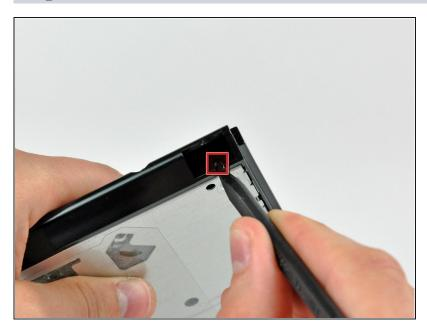
Using the tip of a spudger, press the optical drive bracket tab out of its slot on the side of the optical drive.
