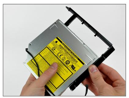
Pull the optical drive bracket toward the open end of the optical drive to free it from the optical drive.
