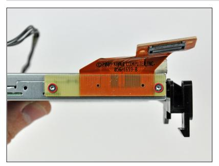
Remove the two T6 Torx screws securing the optical drive cable to the optical drive.
