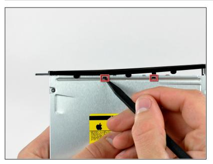
Use the tip of a spudger to press the optical drive bracket tabs out of the slots in the top of the optical drive.
