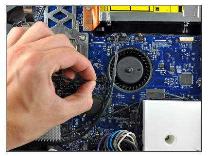
Disconnect the optical drive thermal sensor by pulling its cable toward the left edge of your iMac.
