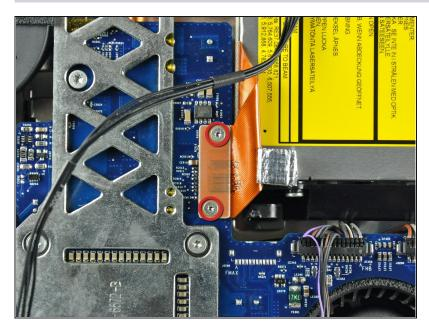
Remove the two T6 Torx screws holding the optical drive connector to the logic board.
