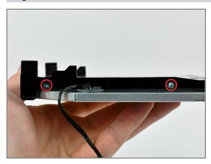
Remove the two T10 Torx screws from the side of your optical drive.
