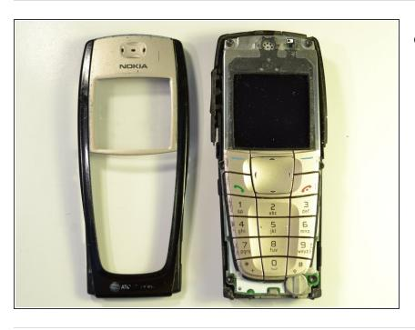
The keypad and LCD screen are revealed.
