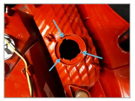
Insert the fitting by matching up the fitting guides with their openings on the casing and turn it 45 degrees clockwise.
