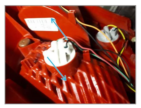
• Unscrew the fitting about 45 degrees and lift it from the casing.
